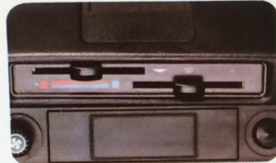
Variable heater/demister control
