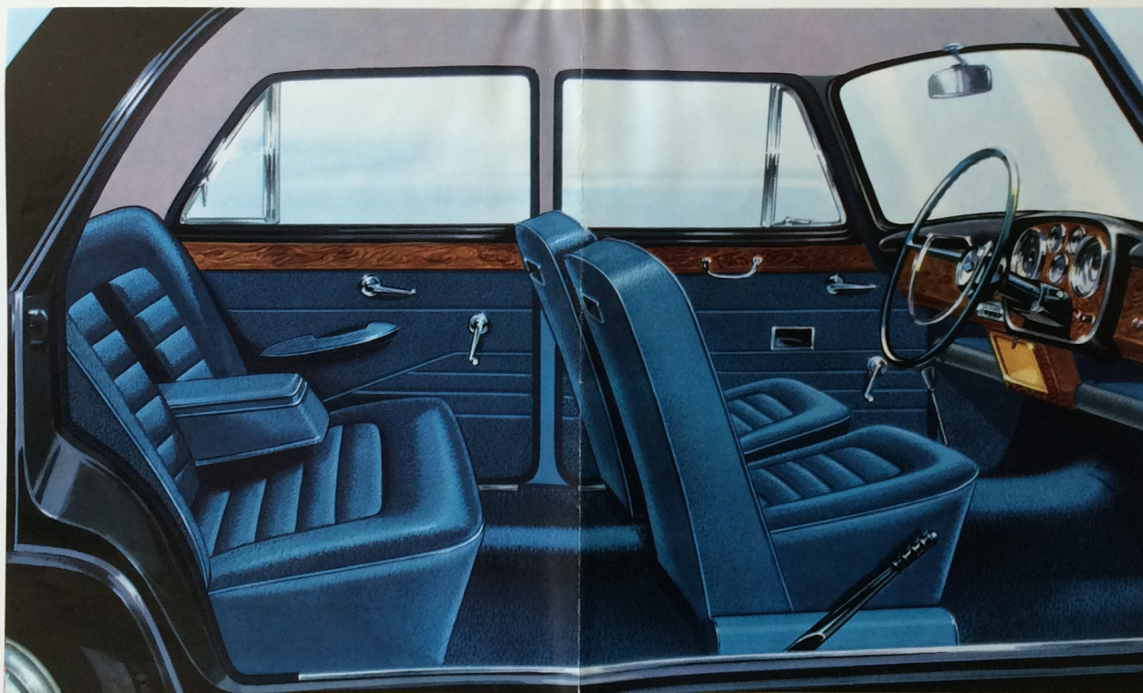
Rich wood fascia with functional and complete instrumentation, including engine revolution counter, fuel and oil pressure gauges, thermometer, ammeter, and electric clock.
